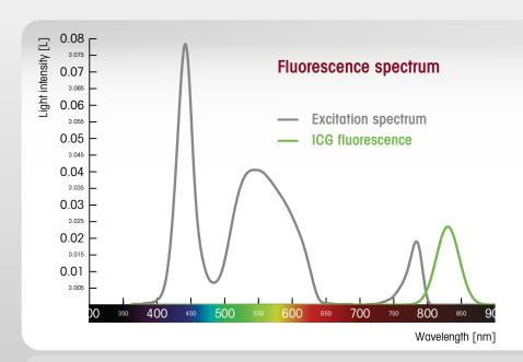
The absorption spectrum of ICG (indocyanine green) is located in the near-infrared range (NIR). Basically ICG absorbs the light in the range of 600 nm to 900 nm and emits the fluorescence between 800 nm up to 850 nm. Thus, it is possible to detect the fluorescence intraoperatively and to visualize with **System green**.
